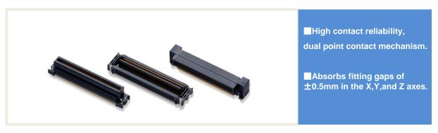
This is a 0.5mm pitch, Board to Board, SMT type connector with a two-point contact mechanism reliability. In case of Iriso's Tandem Contact Connector, the first contact would remove foreign materials (contamination) for better contact reliability. Even if the first contact were on foreign material, the second contact would still be securely touching the contact surface (and vice versa).
