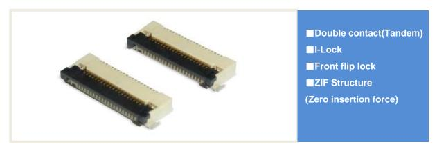
12001 series is 0.5mm pitch SMT, right angle(bottom contact) type FPC/FFC connector. IRISO original "I-Lock" design prevents a dropout of FPC/FFC card and makes good tactile feel to improve workability. Contact is dual contact points system which is good solution for contact contamination by foreign material and flux which contaminate the contacts in the production processes.
